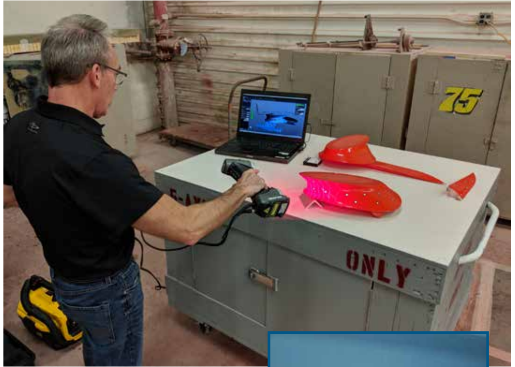
From left: Viking's 3D printer creates a bow thruster tunnel dam for the Valhalla center consoles; Mark Roger's from Viking's New Product Development team works with a portable 3D laser scanner to check the dam's precise dimensions; a completed Valhalla's tunnel with thruster installed.
