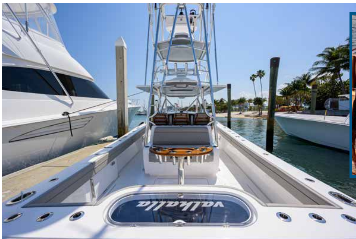
A look forward from the transom shows this V-41's 90-gallon live well with clear lid, its vast array of coaming rod holders and custom teak and stainless cockpit rocket launcher.
