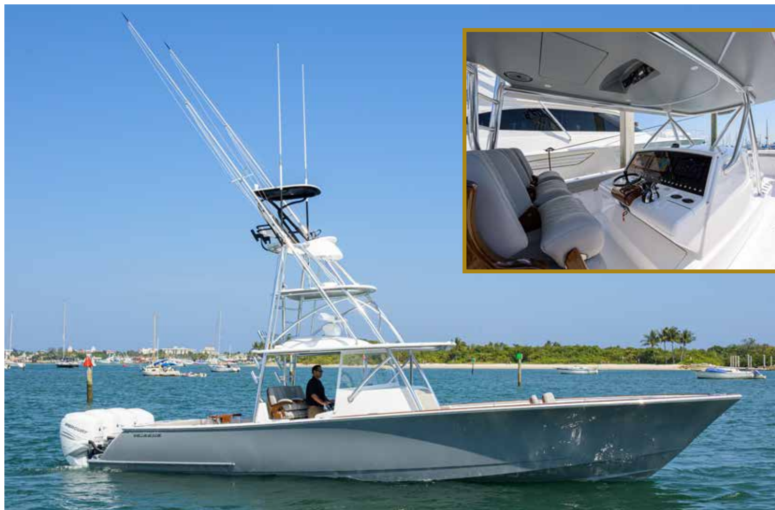
A father and son from south Florida outfitted this V-41 with a custom gap tower. The hardtop features a satin grey underside and recessed locations for electronics, teaser reels and speakers.
