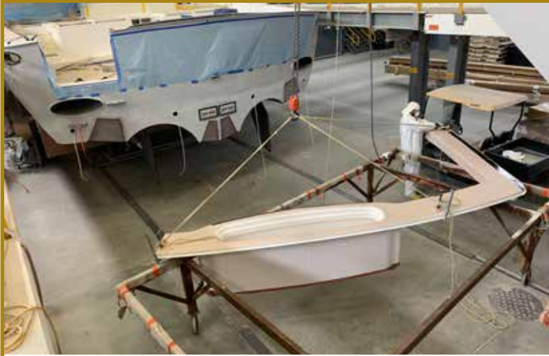
Left: a 92 Convertible's coaming is readied for installation on Line 1. Right: the completed cockpit with teak deck, covering boards and mezzanine.
