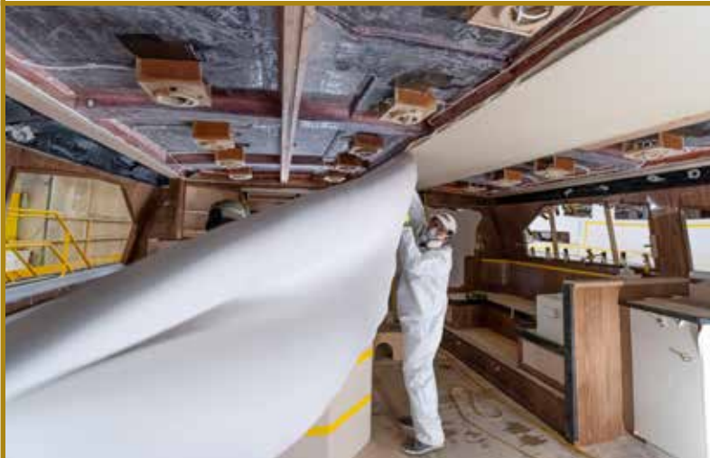
Left: A carpenter installs the headliner in the salon of a 72 Convertible. The square overhead fixtures, or light blocks, that hold the recessed LED lighting are constructed of lightweight materials. Right: The completed salon with all of its beautiful walnut joinery.
