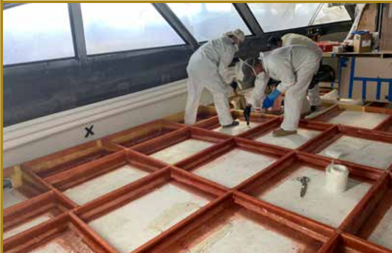
Left: In the enclosed bridge of a 92 Convertible, a team of Carpentry Department shipwrights builds a fiberglass encapsulated grid system that will support the flooring. Right: The 92 EB's appointments include an L-shaped raised lounge, a walnut cocktail table, a 32-inch HD TV, a refrigerator, custom cabinetry and carpeting.
